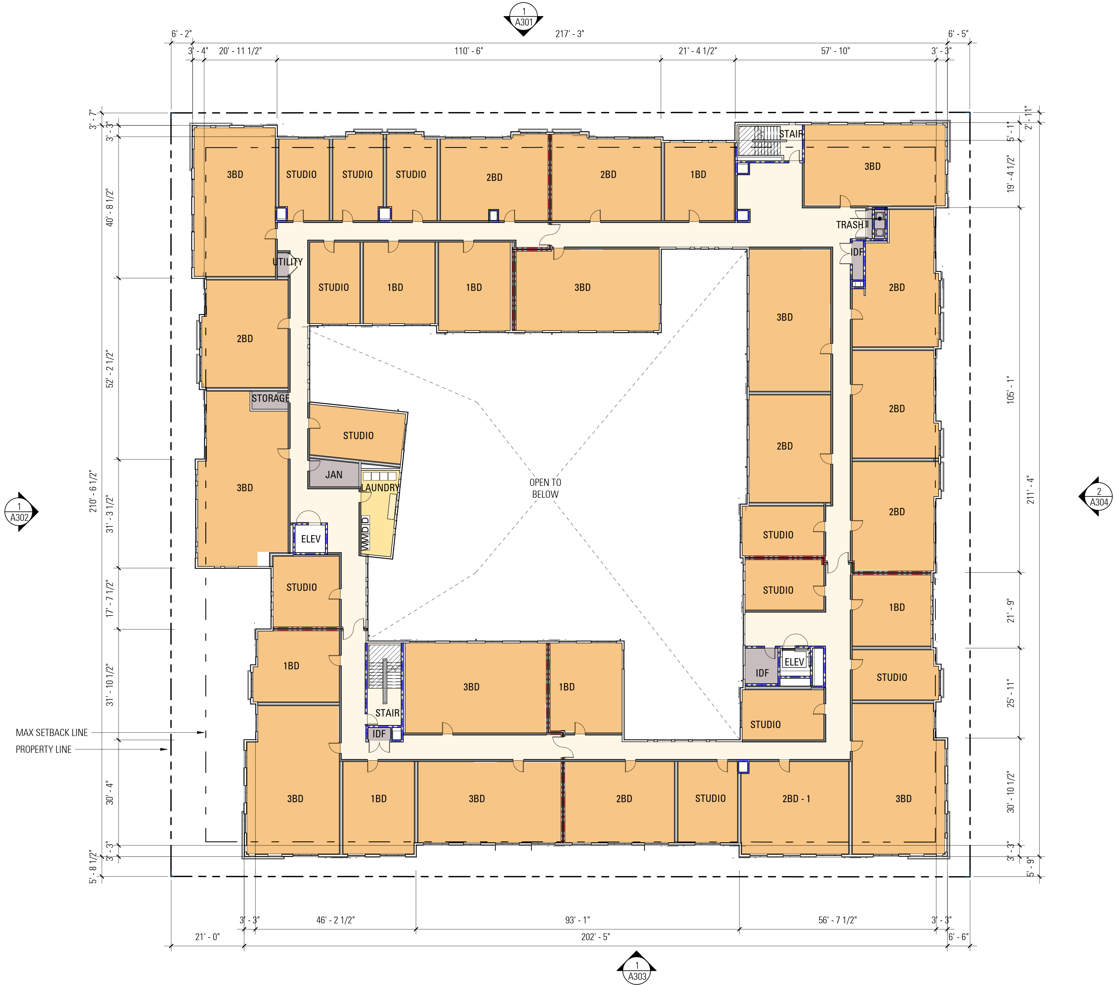
1 A203 FLOOR PLAN - LEVEL 03 - HOUSING BLOCK ENTL 1/16" = 1'-0"
