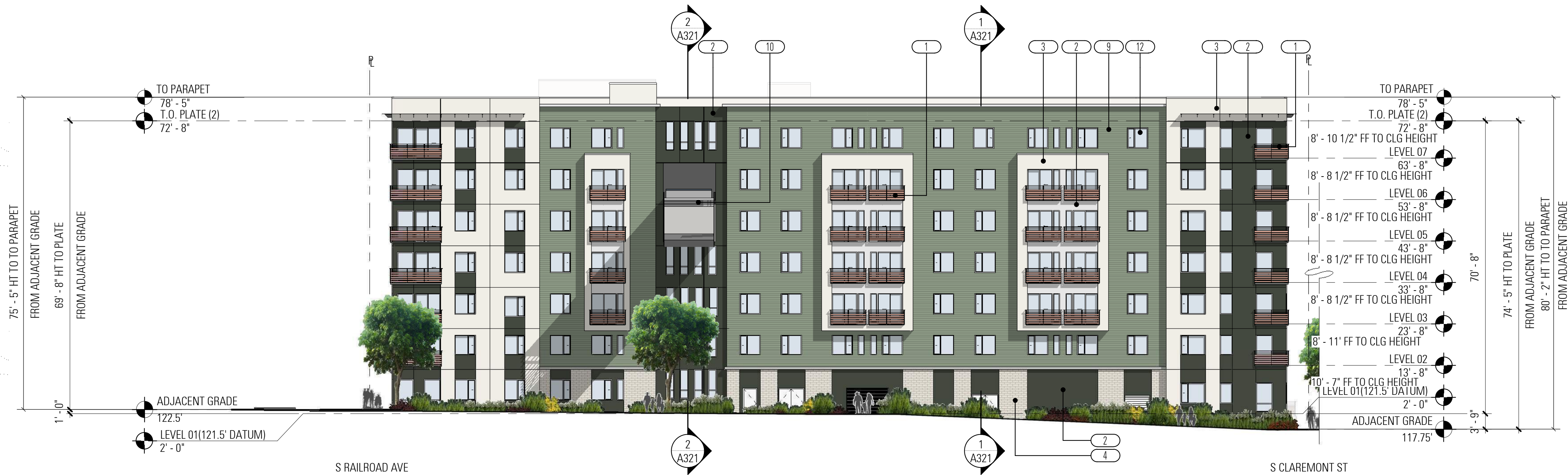
1 A304 EXTERIOR ELEVATION - EAST - HOUSING BLOCK - STREET 1/16" = 1'-0"
