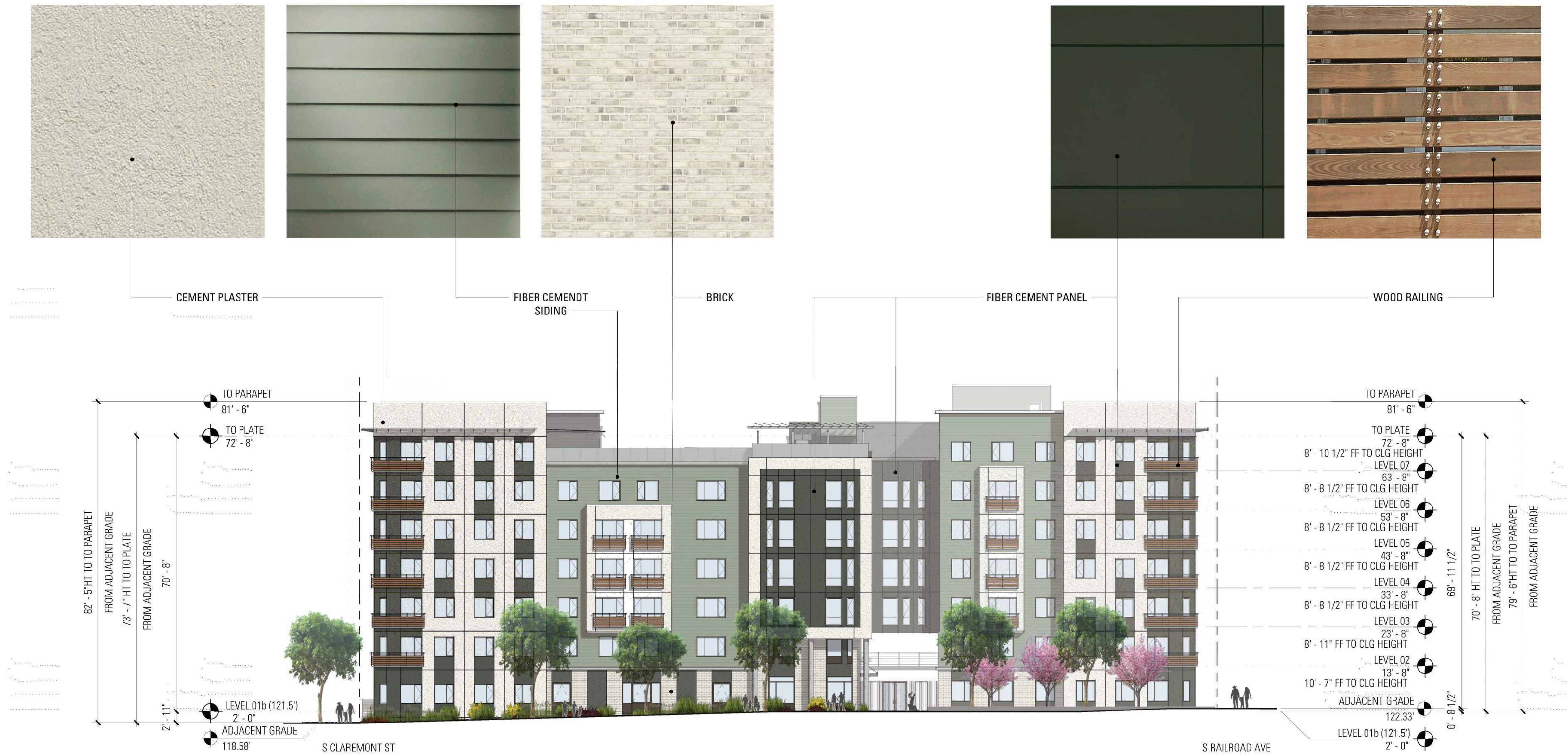
1 A334 EXTERIOR ELEVATION - WEST - EXTERIOR MATERIALS 1/16" = 1'-0"
