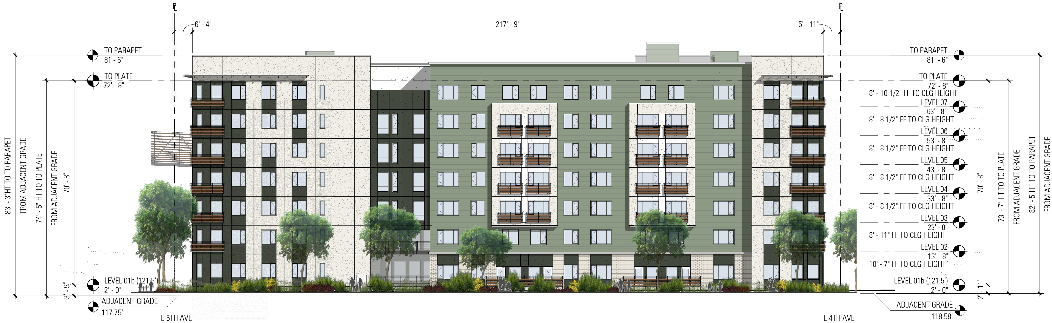
1 A301 EXTERIOR ELEVATION - NORTH - HOUSING BLOCK - STREET 1/16" = 1'-0" AS CURRENTLY PROPOSED
